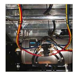
Parflex 1120 Series Tubing is developed for brake system connections that maintain a basically fixed relationship between couplings during vehicle operation. Tubing is made from nylon and is available in more than ten colors for quick identification of lines.
